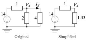
2. [Nodal Analysis] KCL at node  $V_x$  gives  $5 + \frac{V_X}{1} + \frac{V_X}{4} = 0$  which simplifies to  $20 + 5V_X = 0$  from which  $V_X = -4$ .
